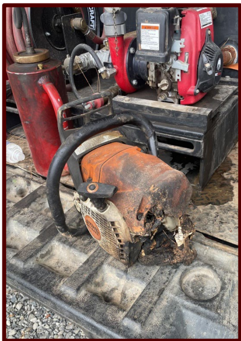
CHAINSAW POWERHEAD AFTER FIRE WAS EXTINGUISHED
